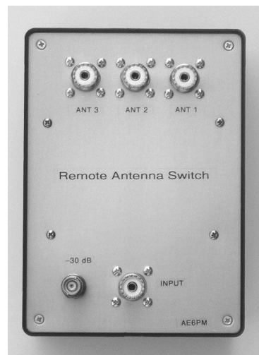
Fig. 1 - My remotely operated 3-position coaxial antenna switch.
